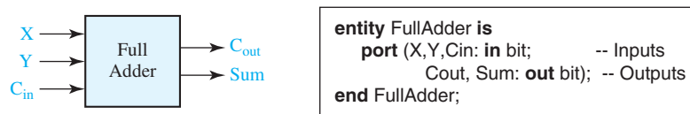
FIGURE 10-10 Entity Declaration for a Full Adder Module
